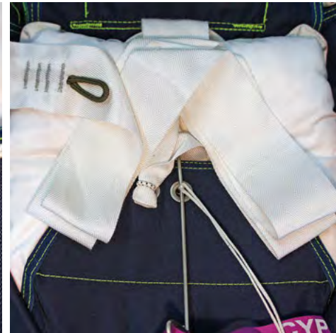
18. Fold bridle in "V" as shown.
