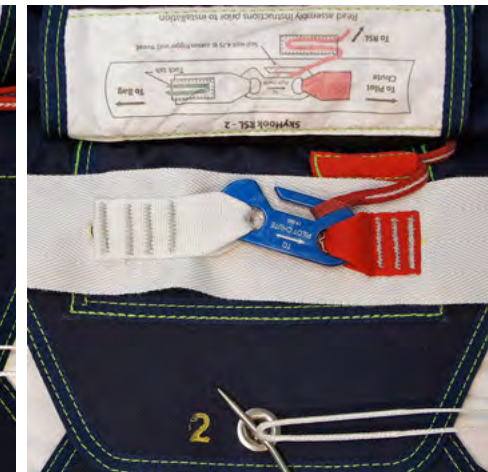
24. Lay the Skyhook bridle over flap #2. Attach the red lanyard to the Skyhook.
