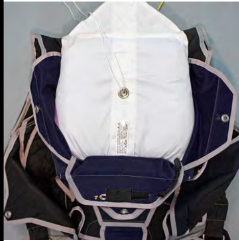
12. Rotate Freebag into reserve container filling lower corners of reserve container.
