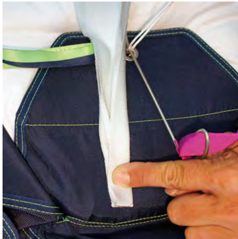
16. Tri-fold reserve bridle lengthwise.
