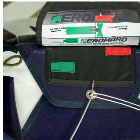
16. Close reserve #2 flap ensuring the bridle exits the left side with green loop exposed.
