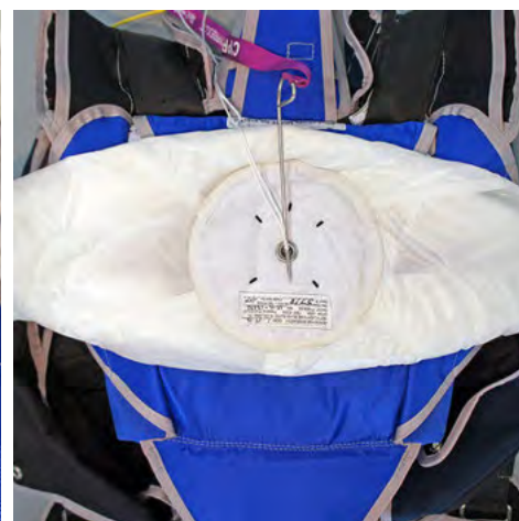
20. Press the pilot chute down into position and hold with a temporary pin. Make sure not to catch the pilot chute fabric under the plate or between the spring coils.
