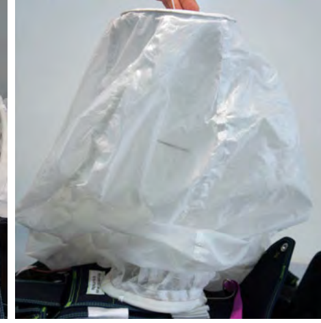
22. Pass the pull up cord cleanly through the pilot chute from bottom to top plate.
