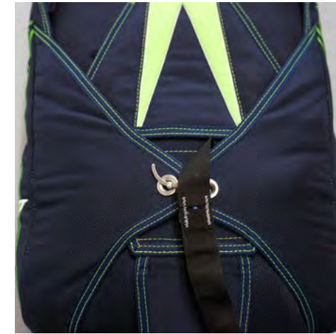
9. Pass the closing loop through grommet on the left side flap (#4), and insert the closing pin.
