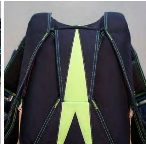
2. Close riser covers over the risers
