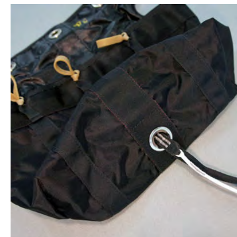
1. Thread the end loop through the D-bag's bottom grommet from the outside until it stops with the confluence wrap.
