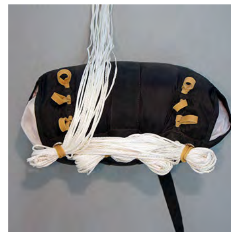
4. Top view stowing the top stows.
