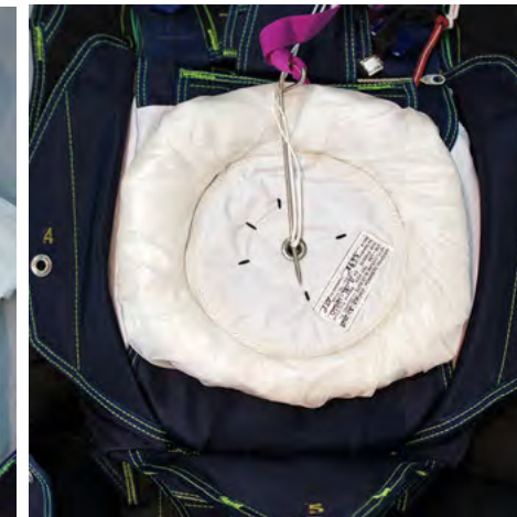
25. Neatly roll the Pilot Chute Fabric up against the outer rim of the Reserve Pilot Chute. Do not tuck the Reserve Pilot Chute Fabric under the lateral closing Flaps #3 and #4.
