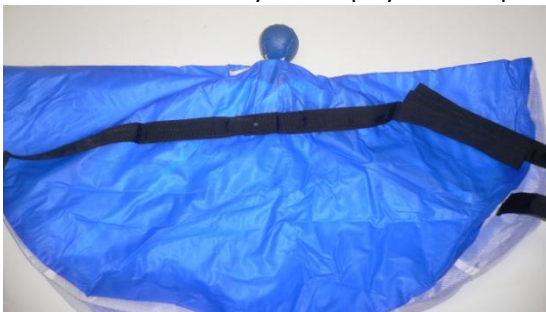
Pilot Chute with hacky sack deploy and collapsible bridle.
