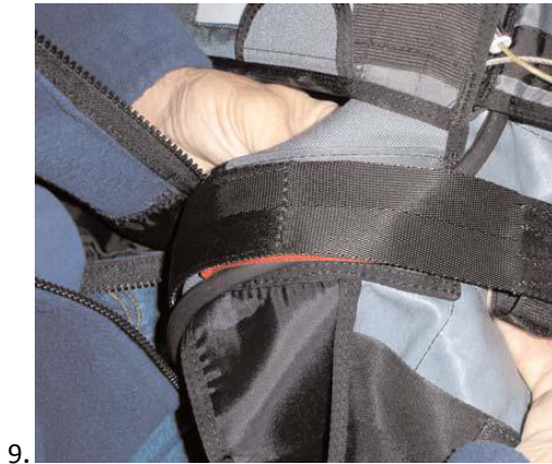
Place Reserve Risers. Ensure Risers are clear from Air Hose.
