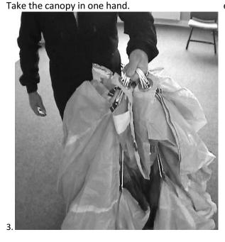
Clear the nose of the canopy by flaking the leading edge. Pull out and count the cells. Align the front edge of the slider with the flaked leading edges.
