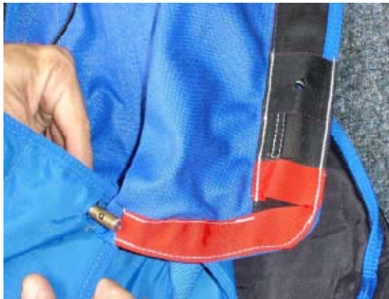
5.1 Thread Cutter thru slit in Panel #1
