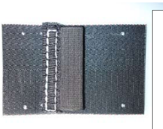
2.5 Stitch Elastic Keeper onto TYPE 12 Webbing as shown. Use Nylon E Thread
