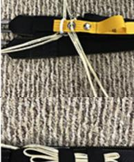
Insert top end of primary toggle (gold toggle) into toggle keeper.
