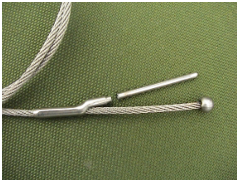
Broken Ripcord Pin
