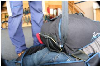
This problem is fixed by extending the fabric over the cable housing.
