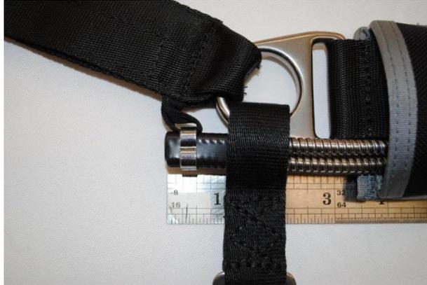
*Photo #4 shows the completed modification with the new position of the heat shrink and the Oetiker clamp.*
