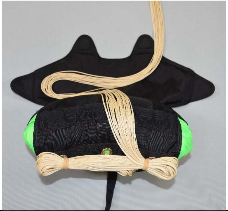
6. Continue folding lines in a figure 8 as shown, with lines extending to both sides of pocket until you have 16" – 20" (40-50cm) of suspension line between bag and connector links.
