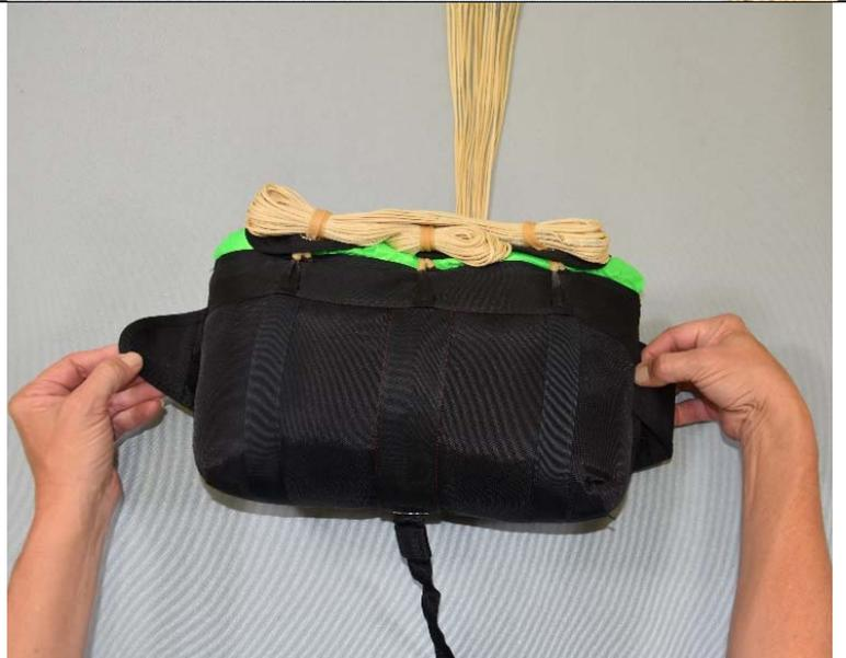
9. Rotate the deployment bag back toward you and tuck magnetic tabs into their magnetic pockets underneath webbing.
