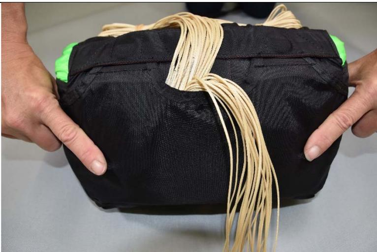
11. Pick up the main deployment bag, securing the lines in the pocket, ensuring the lines do not come out of the pocket while traveling with the bag over harness and into the main tray.
