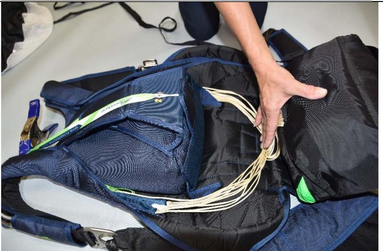
14. Place main deployment bag flat into container with lines stows facing bottom of container and the bridle coming out of the bag towards the bottom of the reserve tray.
