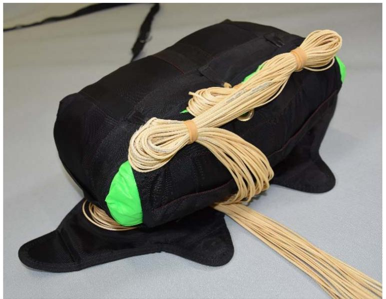
8. Tuck the side tabs into tab pockets on the side of deployment bag.
