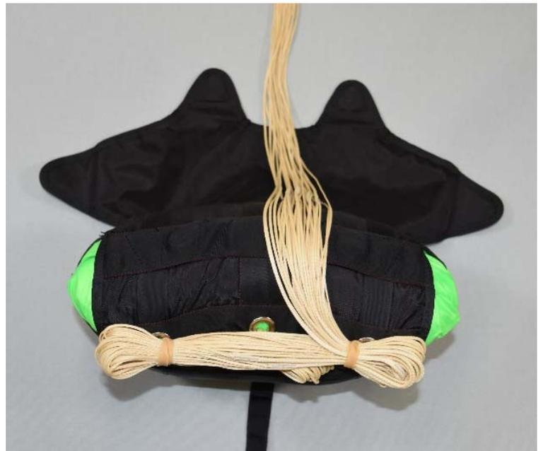
5. Begin to figure 8-fold the suspension line as shown, making sure line groups extend the entire width of the deployment bag.
