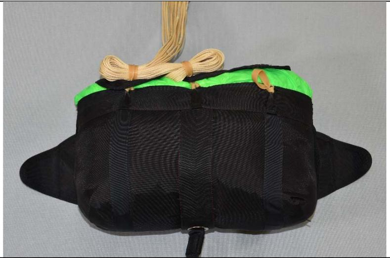
3. Continue stowing all locking stows, using double stows. (Double wrapping large bands around each 2" inch, 5cm line bite)
