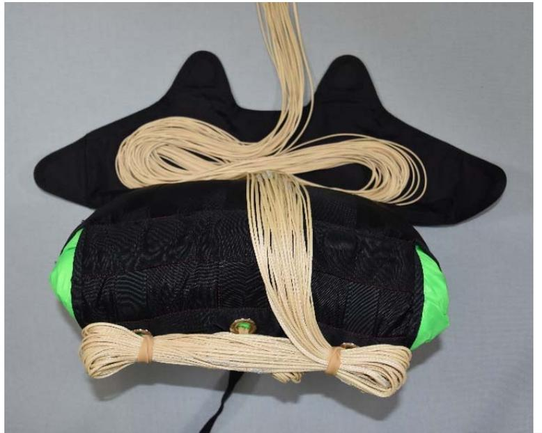
7. Rotate bag toward container, rolling bag onto line stow pocket. Keeping the lines at bottom of line stow pocket.
