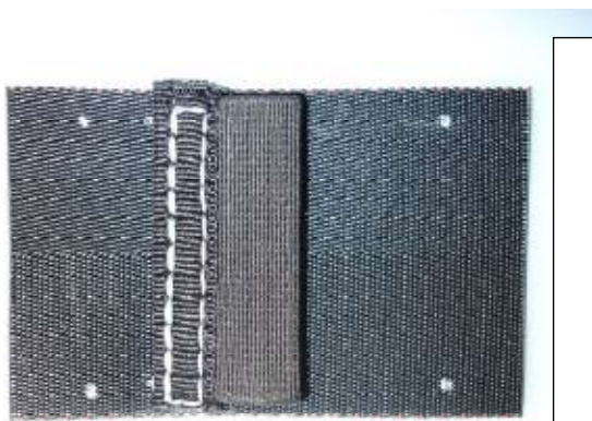
2.5 Stitch Elastic Keeper onto TYPE 12 Webbing as shown. Use Nylon E Thread
