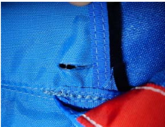
4.10 Use a hot knife and cut 15mm slot in Flap #1 as shown
