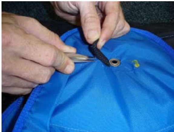
1.5 Carefully unpick Elastic Keeper. Elastic Keeper is reused
