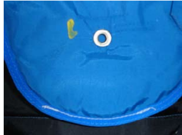
1.6 Rebind. Reserve Flap #1 is complete. Binding stitch shown in white. Back tack at least 10mm
