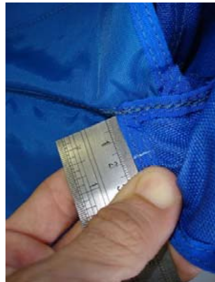
4.2 Measure and mark 20mm from Intersection between Flap #1 and Flap #2. This mark is the alignment mark for the start of the tunnel
