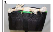
Center locking stows are to be made before moving along to the outer locking stows. All locking stows are to be free and clear of each other.
