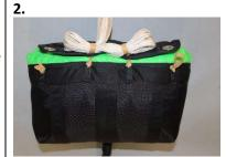
Insert canopy into the main deployment bag. Starting with the center, route the large packing rubber bands through the corresponding grommet and secure line bite approximately 1.5-2" inches in length using the double stow method.
