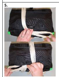
Continue figure 8 line placement into magnetic line stow pocket, ensuring line stows are as wide as line stow pocket.
