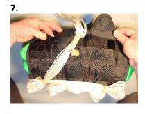
Close magnetic line stow pocket by inserting magnetic tuck tabs into their magnetic pockets <u>underneath</u> black webbing.
