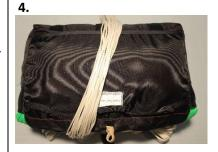
Route the excess suspension line over top of bag down to the bottom of line stow pocket.
